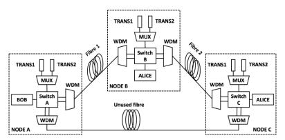
Figure 12-11: Diagrammatic description of the testbed used to implement the use-case in 2018
