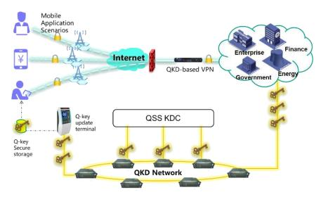
Figure 11-3: QKD-key embedded secure mobile communication
