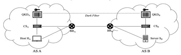
Figure 12-17: High-level overview of the SCION-QKD integration model
