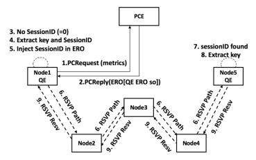
Figure 12-12: MPLS/PCEP workflow for setting up a quantum encryption service
