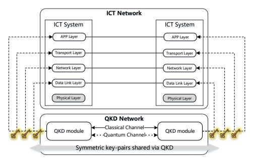
Figure 9-1: QKDN integrated with TCP/IP protocol stack
